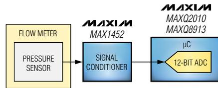
Figure 2. Typical front-end for a pressure sensor.
