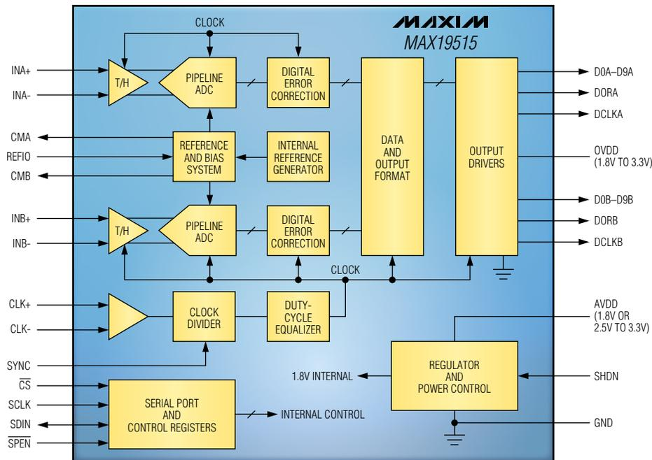
Typical operating circuit for the MAX19515, which detects high-speed pulse signals.
