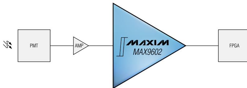
*An ultra-high-speed MAX9602 comparator is used in a basic PET system to detect precise time-of-flight information.*
