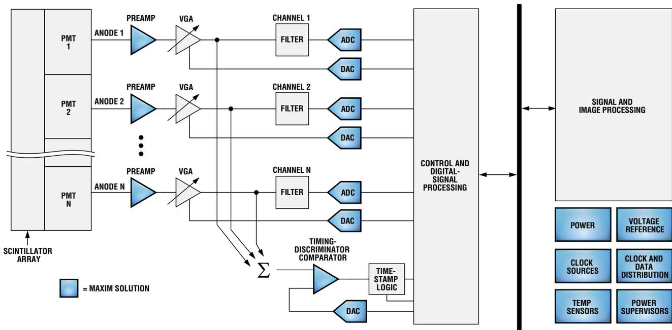
Block diagram of a PET system. This diagram shows one of multiple receiver groups that share a common time discriminator. For a list of Maxim's recommended PET solutions, please go to: [www.maxim-ic.com/pet](http://www.maxim-ic.com/pet).
