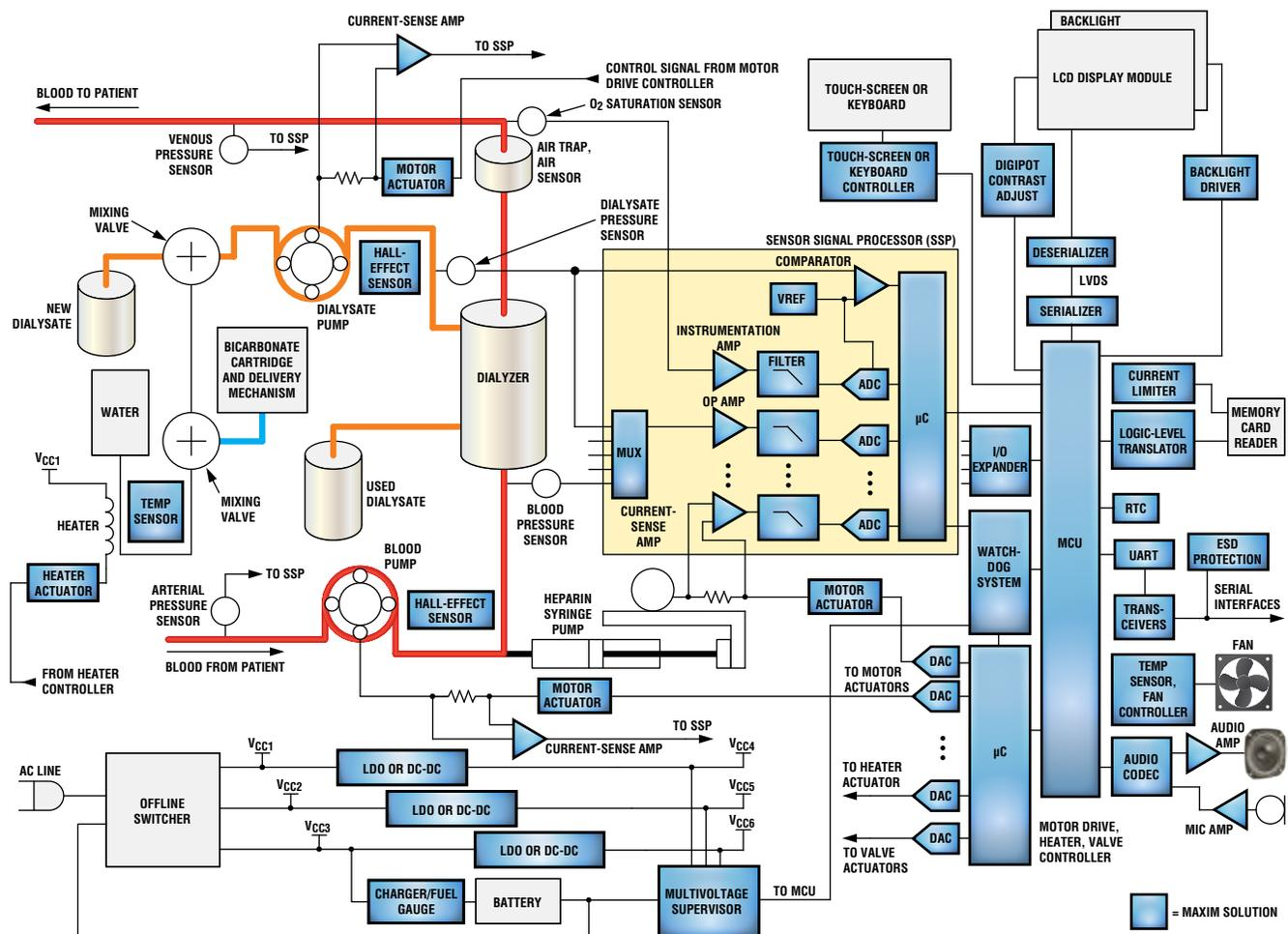
Block diagram of a home-use dialysis machine. For a list of Maxim's recommended solutions for dialysis machines, please visit: [www.maxim-ic.com/dialysis](http://www.maxim-ic.com/dialysis).
