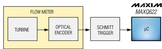
Figure 1. Typical front-end for a turbine transducer.
