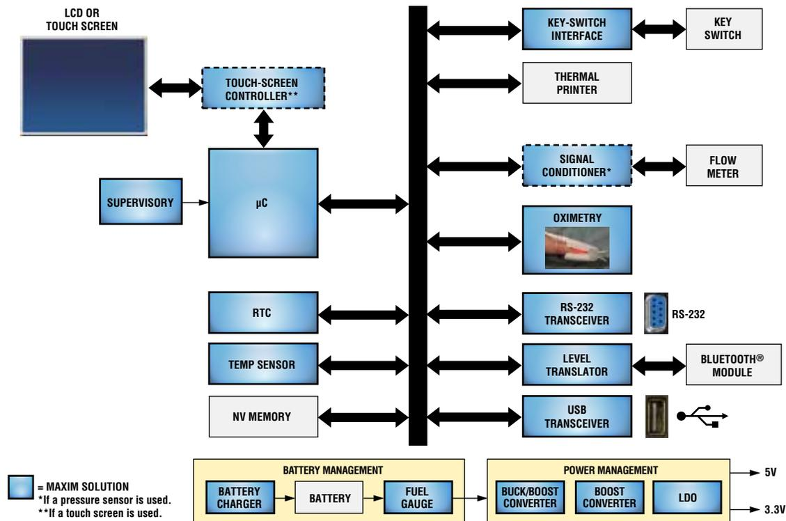
System block diagram of a desktop spirometer. For a list of Maxim's recommended solutions for spirometers, please visit: [www.maxim-ic.com/spirometer](http://www.maxim-ic.com/spirometer).
