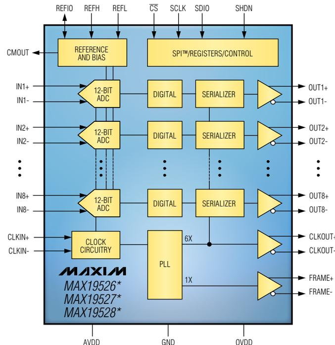
Typical operating circuit for the MAX19526/MAX19527/MAX19528.
