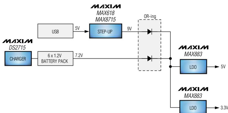
Figure 3. Power-supply example for a desktop spirometer.
