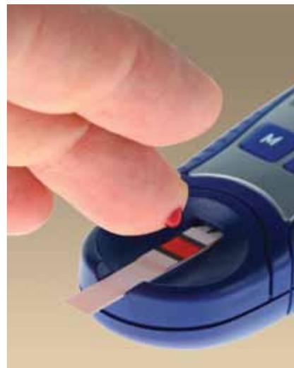
*Optical-reflectometry blood glucose meter*
