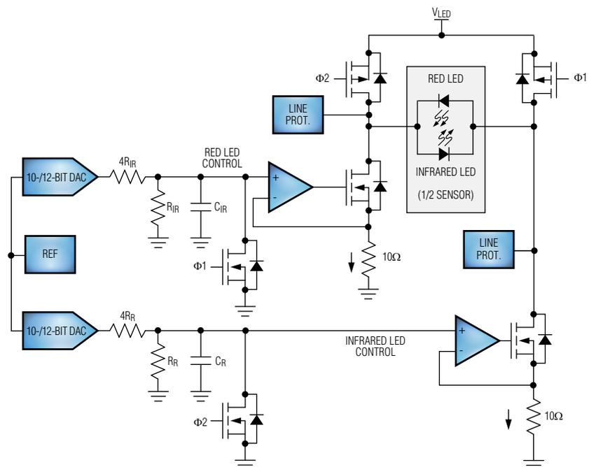
Figure 1. Simplified red and infrared LED bias and control circuit.
