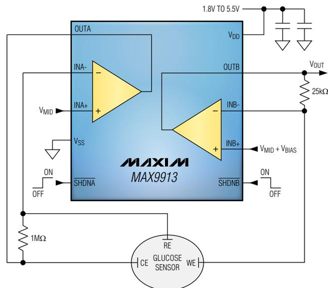
MAX9913 in a three-electrode, electrochemical glucose meter application.
