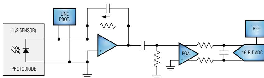
Figure 2. Simplified photodiode receive path circuit.
