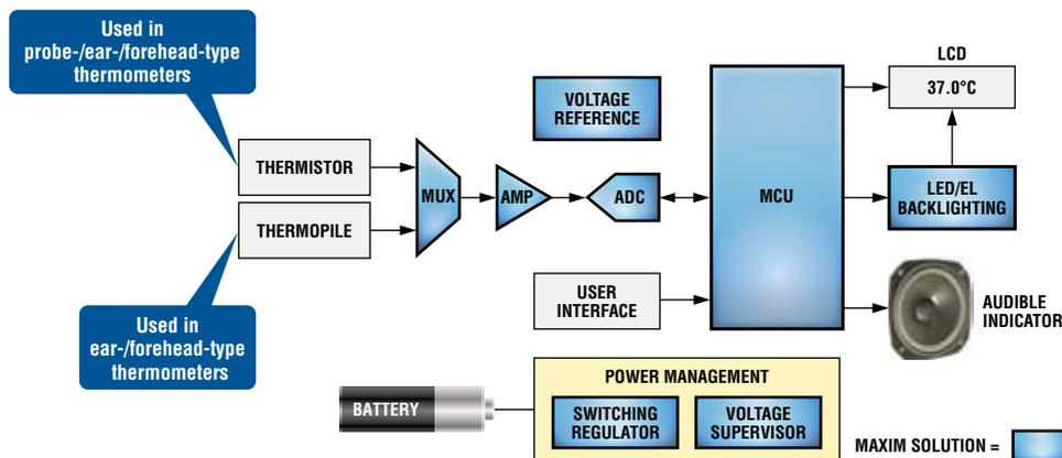
Functional block diagram of a digital thermometer. For a list of Maxim's recommended solutions for digital thermometer designs, please go to: [www.maxim-ic.com/thermometer](http://www.maxim-ic.com/thermometer).
