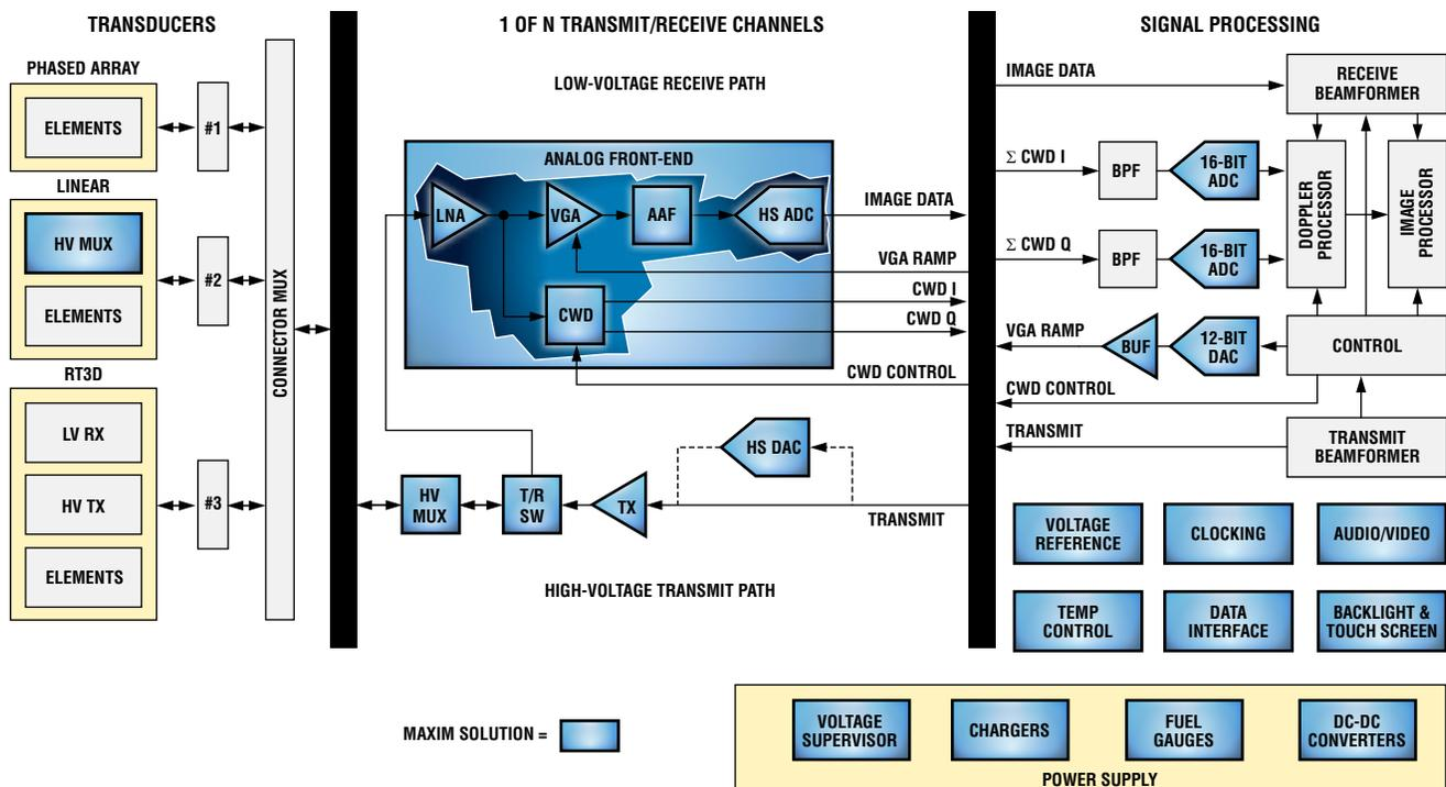
Functional block diagram of an ultrasound imaging system. For a list of Maxim's recommended ultrasound solutions, please go to: [www.maxim-ic.com/ultrasound](http://www.maxim-ic.com/ultrasound).
