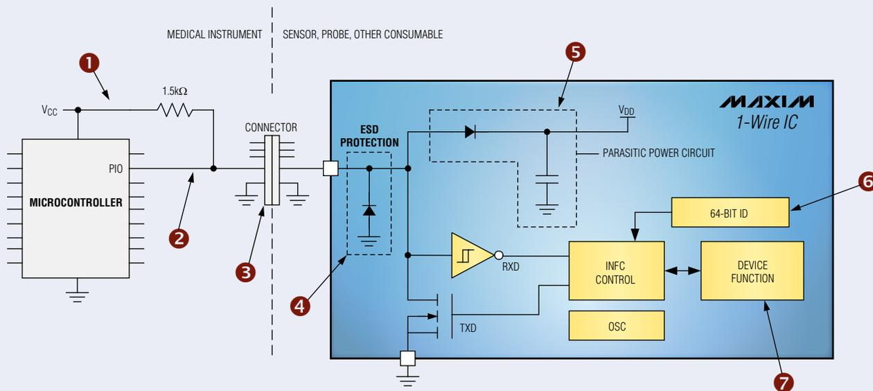
Typical interface from a medical instrument to a 1-Wire device.
