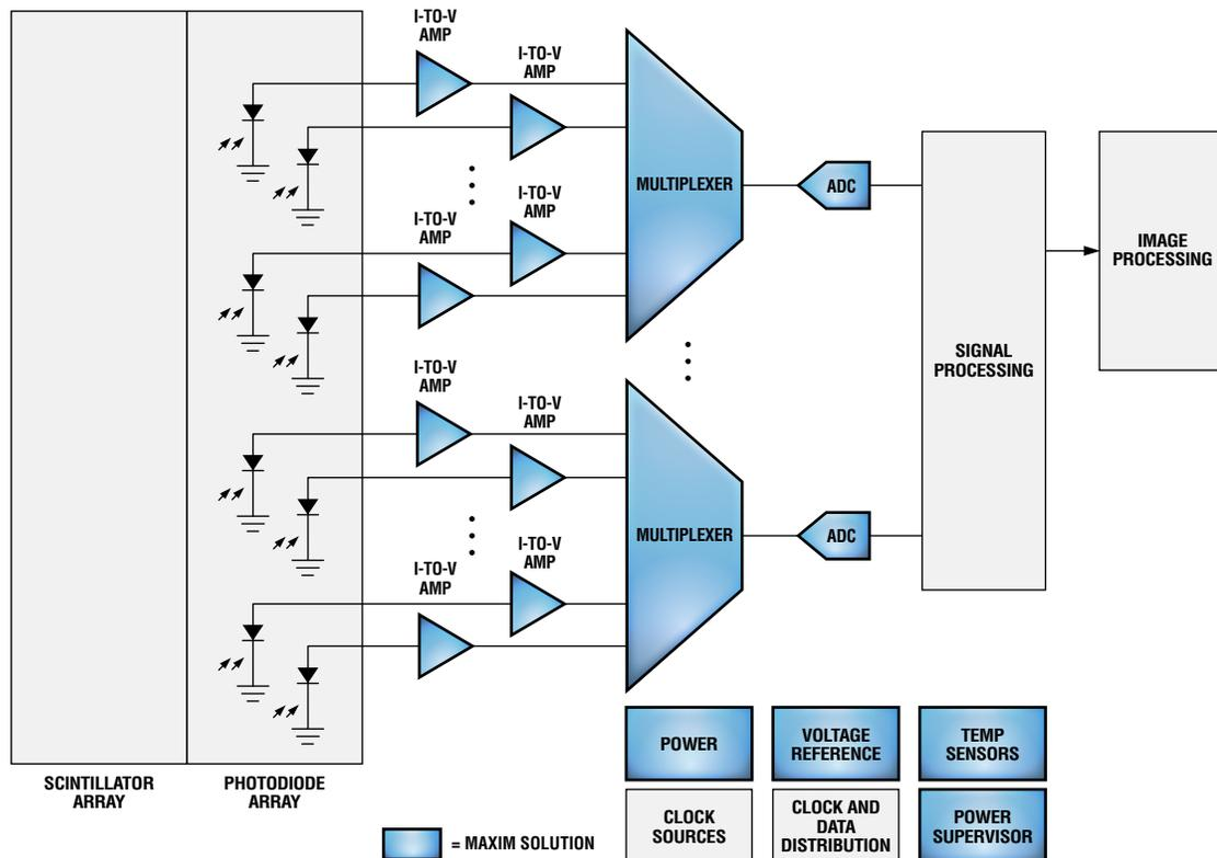
Block diagram of a CT imaging system. For a list of Maxim's recommended CT imaging solutions, please go to: [www.maxim-ic.com/ct](http://www.maxim-ic.com/ct).
