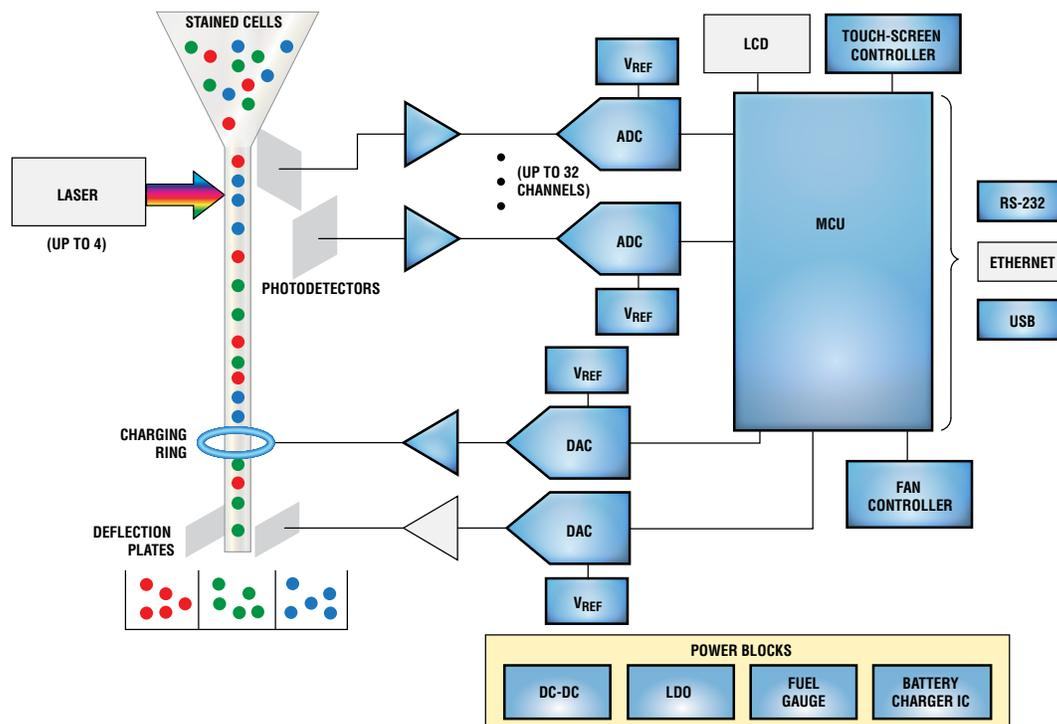
System block diagram for a flow cytometer. For a list of Maxim's recommended solutions for flow cytometers, go to the solutions page below.
