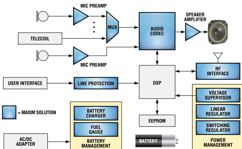
Digital hearing aid functional block diagram. For a list of Maxim's recommended solutions for hearing aid designs, please go to: [www.maxim-ic.com/hearing](http://www.maxim-ic.com/hearing).
