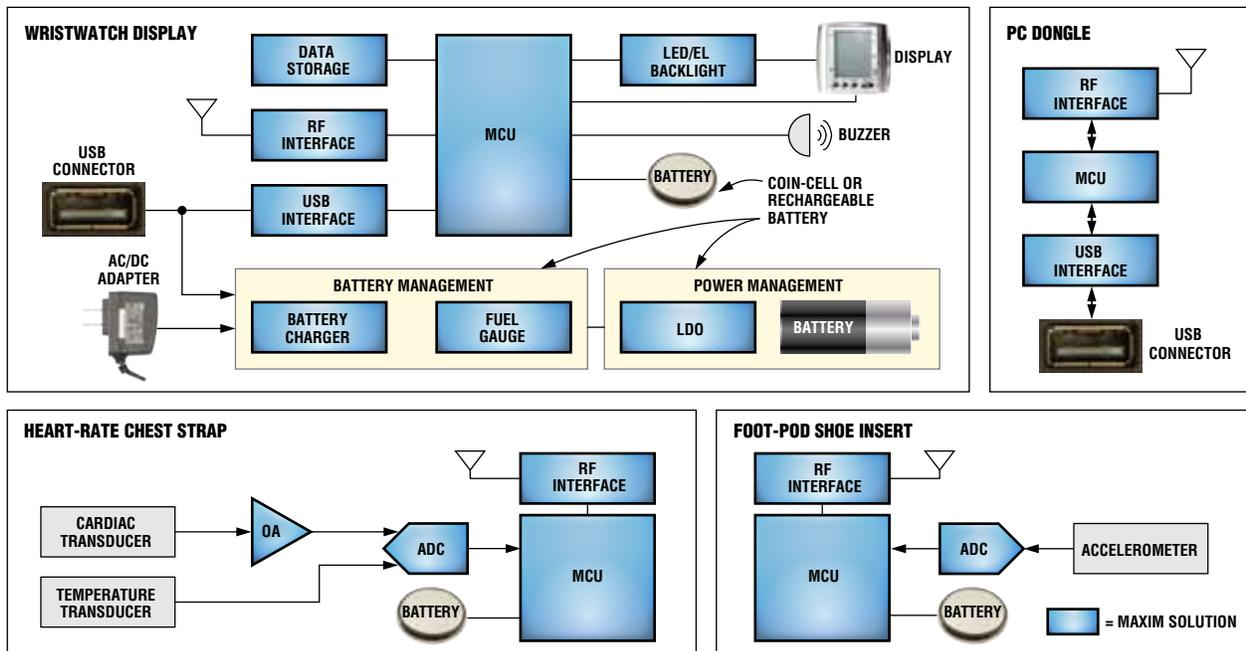
Functional block diagram of a heart-rate/fitness monitor. For a list of Maxim's recommended solutions for heart-rate/fitness monitors, go to the solutions page below.
