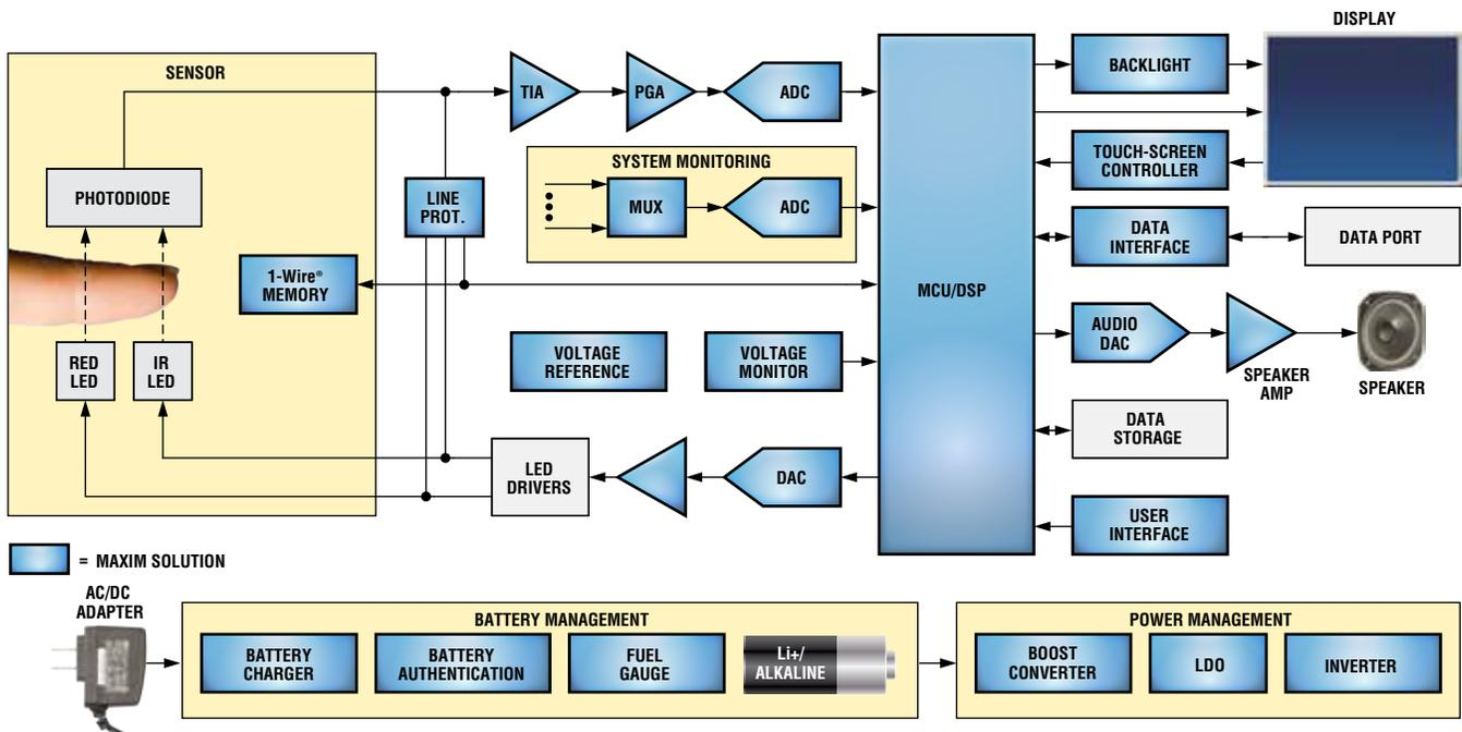
Functional block diagram of a pulse oximeter. For a list of Maxim's recommended solutions for pulse oximeters, please go to: [www.maxim-ic.com/pulseox](http://www.maxim-ic.com/pulseox).
