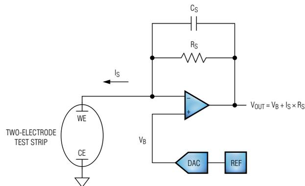
Figure 1. Electrochemical test strip in a self-biased configuration.
