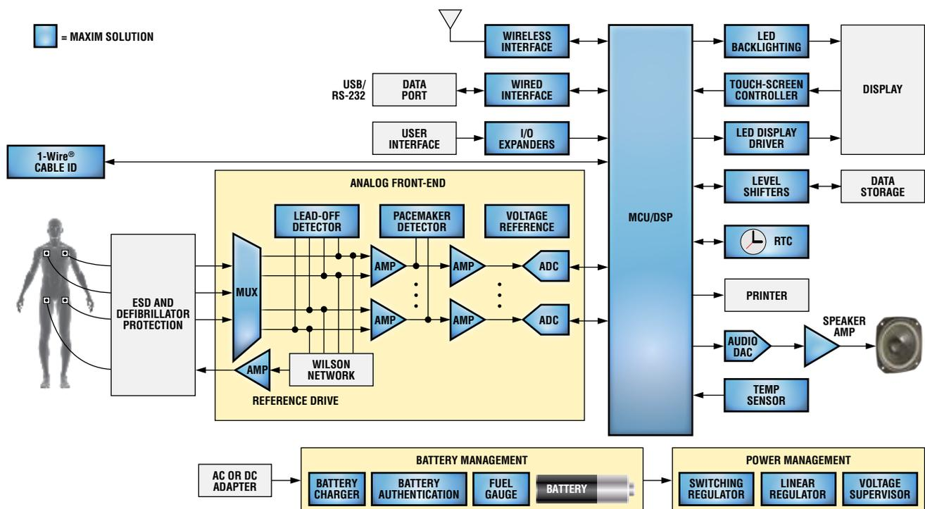
Full-featured ECG functional block diagram. For a list of Maxim's recommended solutions for an ECG design, please go to: [www.maxim-ic.com/ECG](http://www.maxim-ic.com/ECG).
