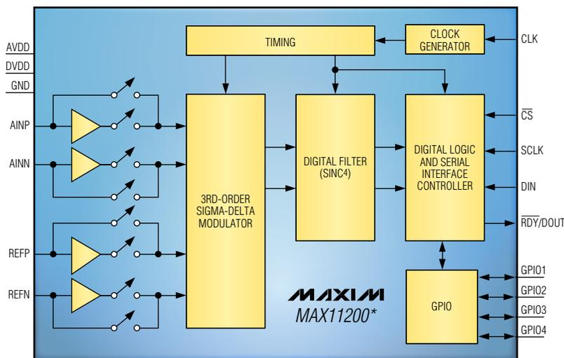
The MAX11200's integrated GPIOs allow control of an external 16-channel mux without needing additional isolation components.
