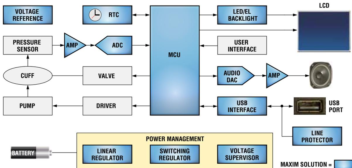
Functional block diagram of a blood pressure monitor that includes an advanced voice indicator. For a list of Maxim's recommended solutions for blood pressure monitor designs, please go to: [www.maxim-ic.com/bloodpressure](http://www.maxim-ic.com/bloodpressure).
