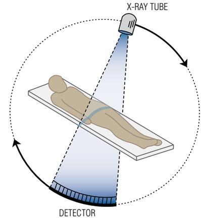
The patient is exposed to a fan-shaped x-ray beam, and the projected image is detected on a thin, semicircular digital x-ray detector.
