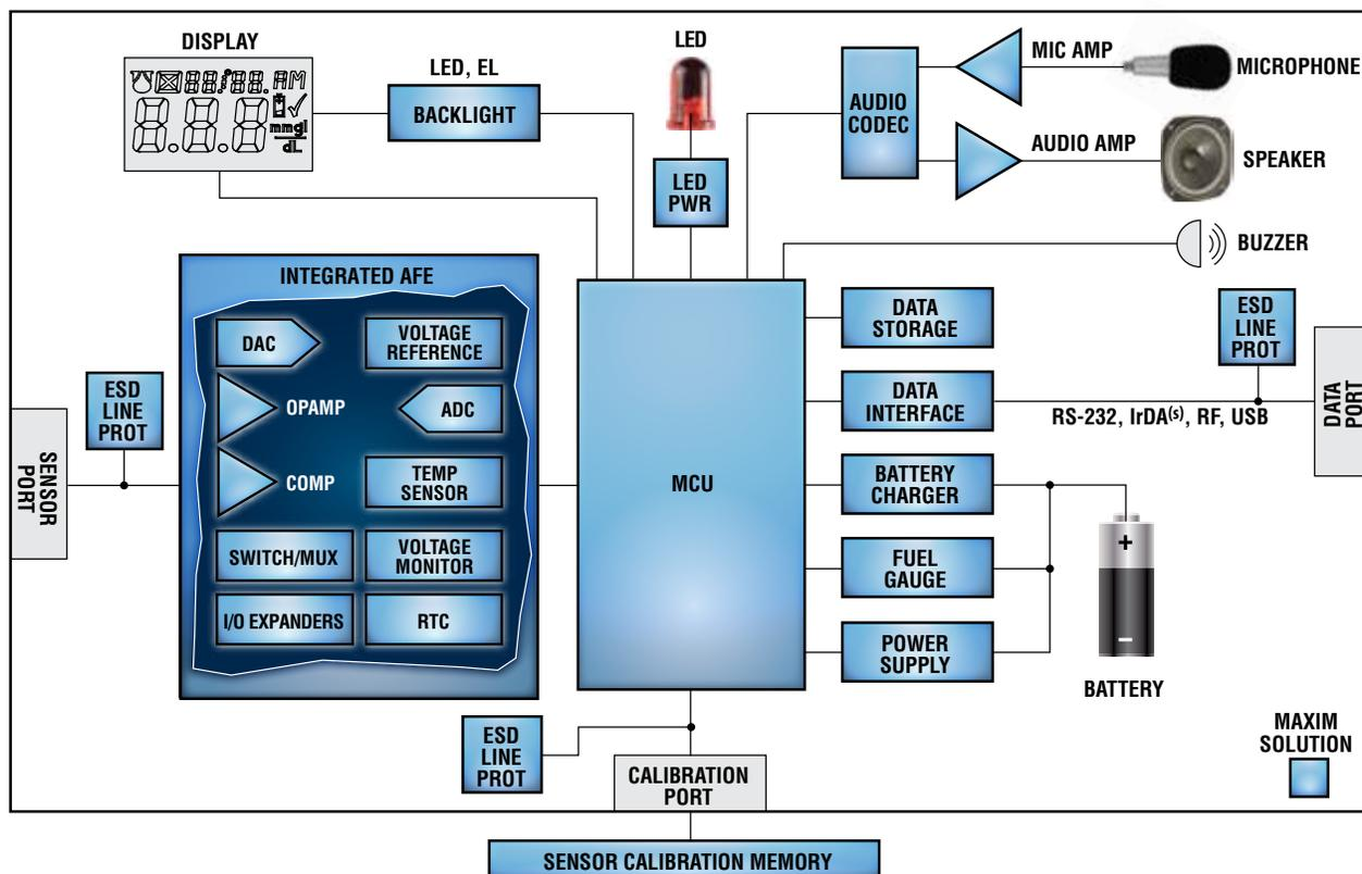
Functional block diagram of a blood glucose meter. For a list of Maxim's recommended glucose-meter solutions, please go to: [www.maxim-ic.com/glucose](http://www.maxim-ic.com/glucose).
