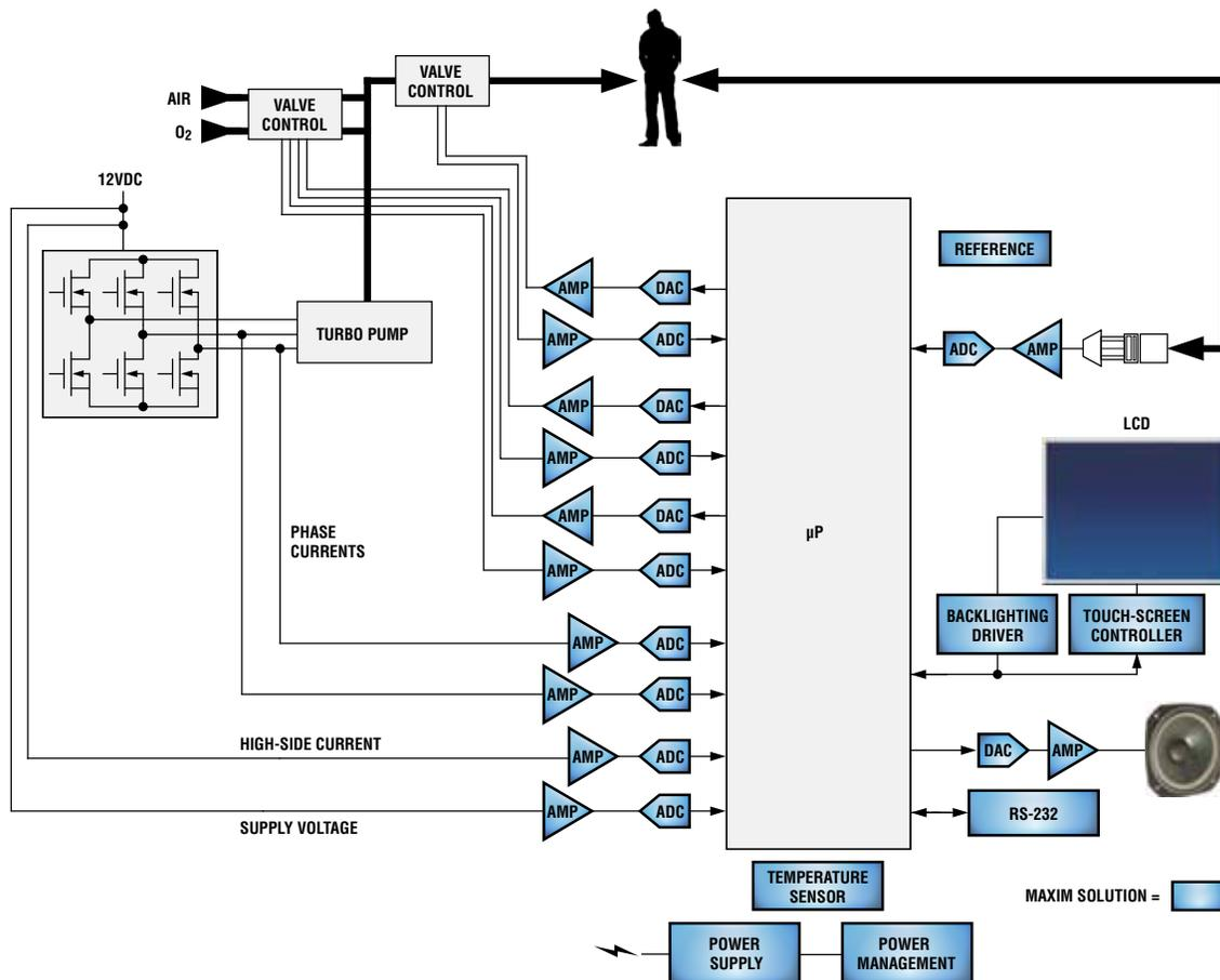
Functional block diagram of a ventilator system. For a list of Maxim's recommended solutions for ventilator designs, please go to [www.maxim-ic.com/ventilator](http://www.maxim-ic.com/ventilator).
