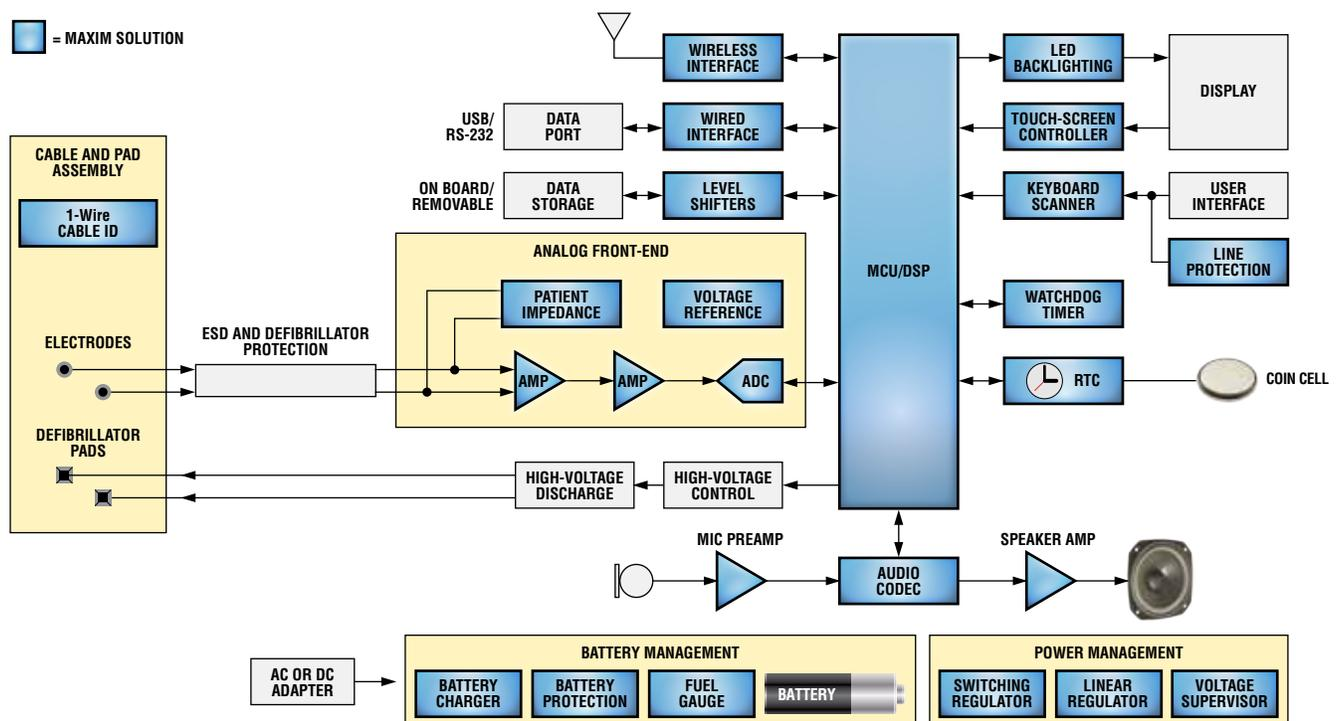
Functional block diagram for an AED device. For a list of Maxim's recommended solutions for an AED design, please go to: [www.maxim-ic.com/ECG](http://www.maxim-ic.com/ECG).
