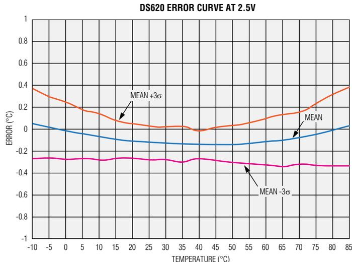
*The DS620's low temperature-measurement error helps ensure instrument accuracy.*
