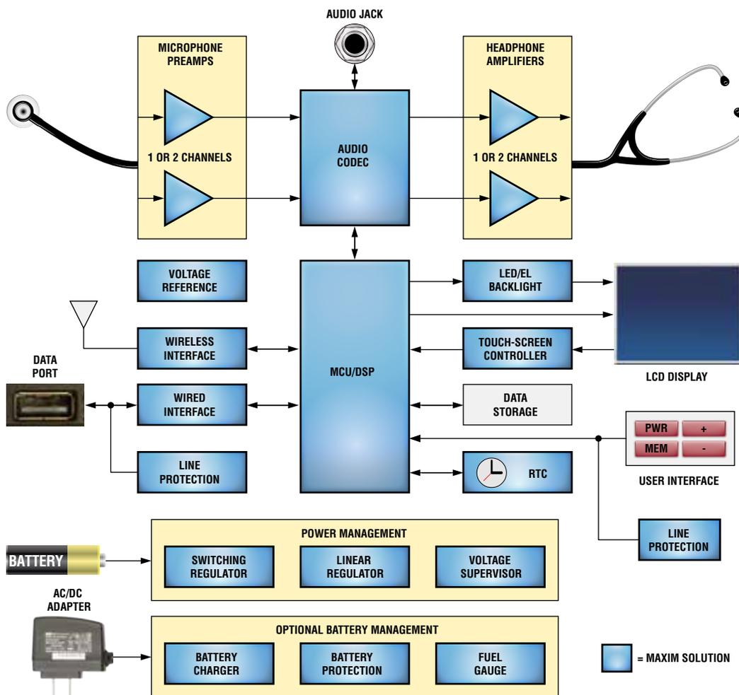
Functional block diagram of a digital stethoscope. For a list of Maxim's recommended digital-stethoscope solutions, please go to: [www.maxim-ic.com/stethoscope](http://www.maxim-ic.com/stethoscope).
