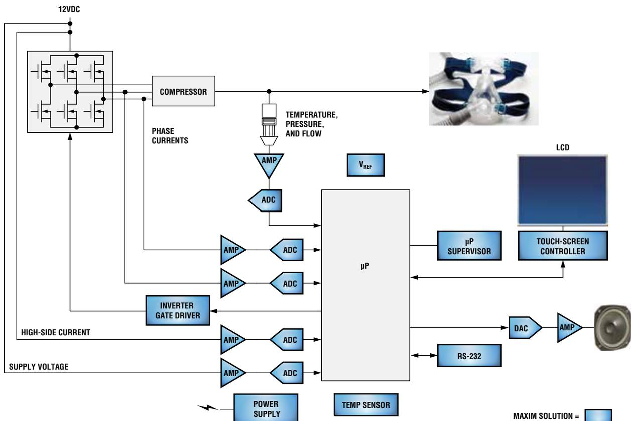
Functional block diagram of a CPAP system. For a list of Maxim's recommended solutions for CPAP designs, please go to: [www.maxim-ic.com/CPAP](http://www.maxim-ic.com/CPAP).
