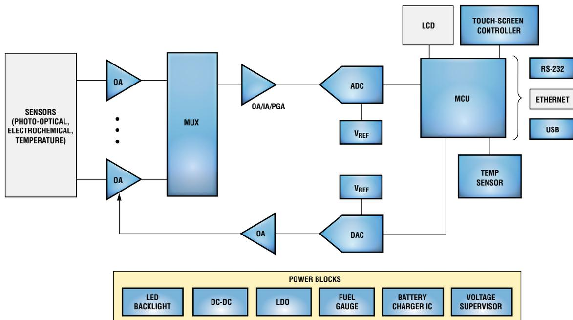
OA = Operational Amplifier, IA = Instrumentation Amplifier, PGA = Programmable Gain Amplifier
