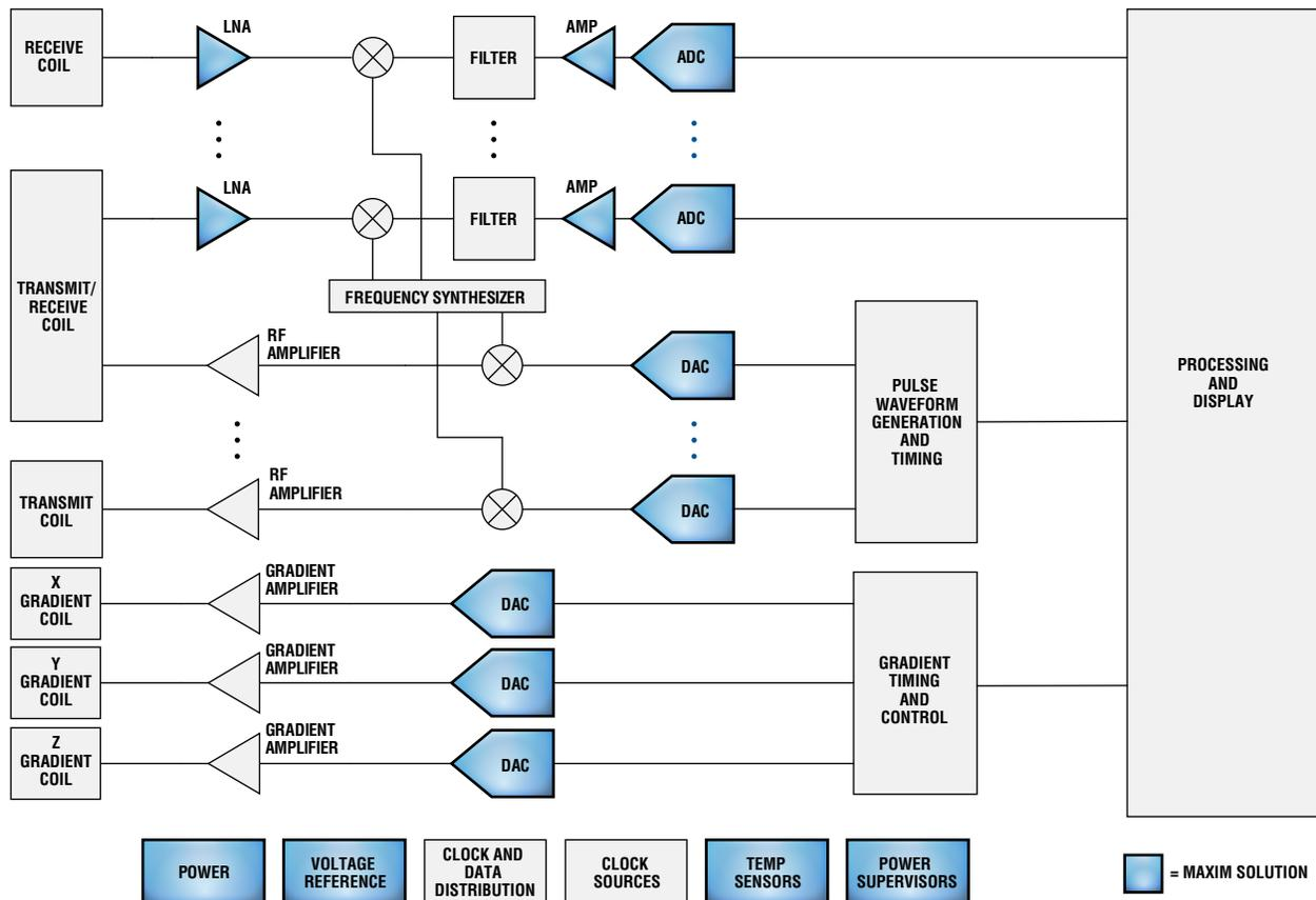
Block diagram of an MRI imaging system. For a list of Maxim's recommended MRI solutions, please go to: [www.maxim-ic.com/mri](http://www.maxim-ic.com/mri).
