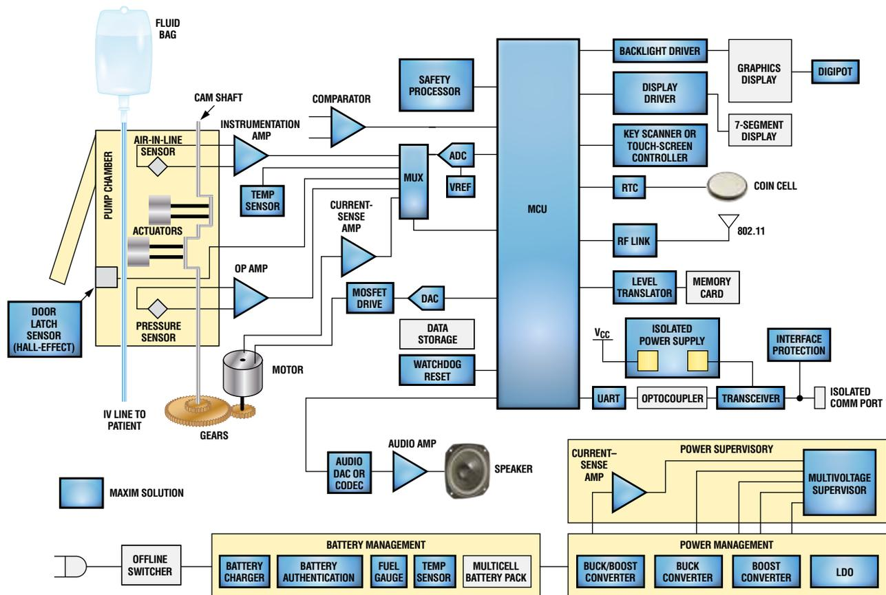
Functional block diagram of an infusion pump. For a list of Maxim's recommended solutions for infusion pumps, please visit: [www.maxim-ic.com/infusion](http://www.maxim-ic.com/infusion).
