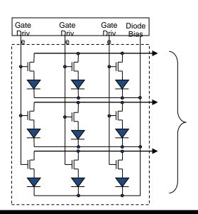
multiplexed photodiode outputs to readout electronics
