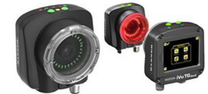
Figure 6: Image sensors from the iVu series can identify workpieces by type, size, location, orientation, and coloring. The machine-vision components can accept configuration and monitoring an integrated screen, remote HMI, or PC. Camera, controller, lens, and light are all pre-integrated. Image source: Banner Engineering Corp.
