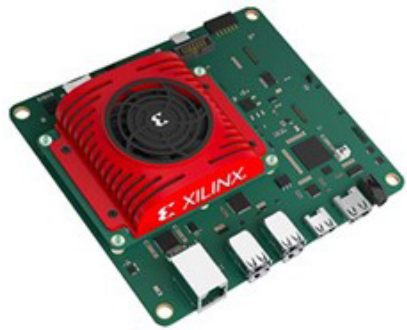
Figure 5: The Kria KV260 vision AI starter kit is a comprehensive development environment for machine vision applications. Image source: AMD Xilinx
