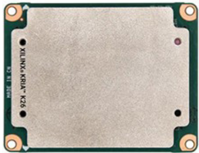
Figure 7: Production-optimized Kira 26 SOMs for industrial and commercial environments are designed to be plugged into a carrier card with solution-specific peripherals. Image: DigiKey
