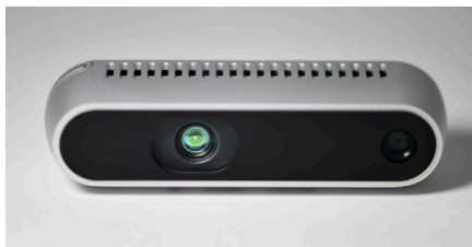
Figure 9: Intel RealSense D435f depth camera Credit: Intel Corporation
