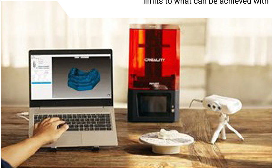
Figure 4: 3D scanners capture 2D images of an object to create a 3D model of it. In some cases, the digital models are then employed to 3D print copies. Image source: Shenzhen CreaLity 3D Technology Co.
