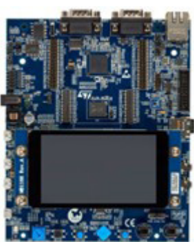
Figure 4: The STM32H757I-EVAL board provides developers with lots of expansion space, easy access to peripherals, and an LCD screen to get started with multicore applications. Image source: STMicroelectronics
