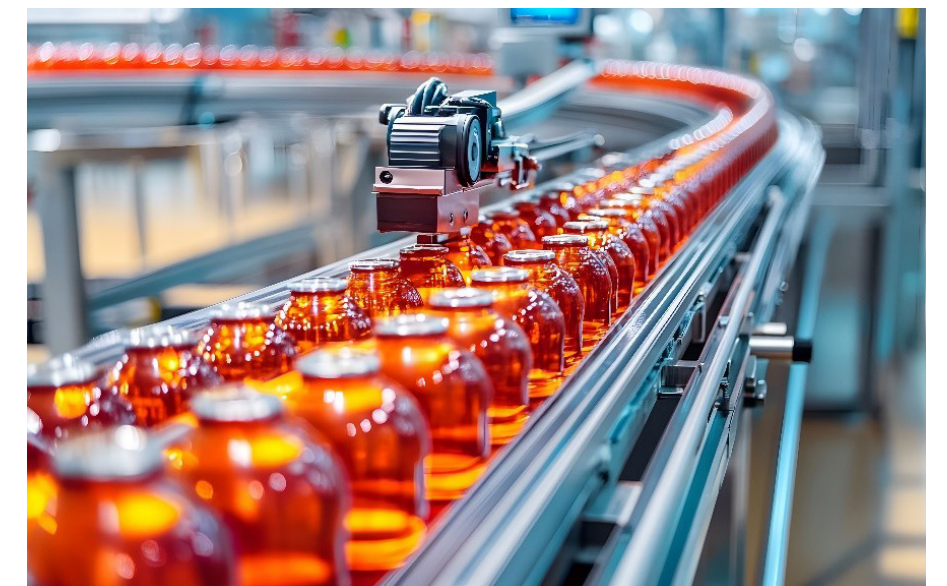
Figure 2: Camera performing 360° inspection of products on a conveyor
