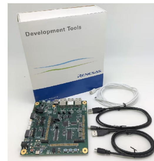
Figure 5: The RTK9RZN2L0S00000BE Starter Kit+ includes the necessary hardware and software, plus application examples, to support development of deterministic networking. Image source: Renesas
