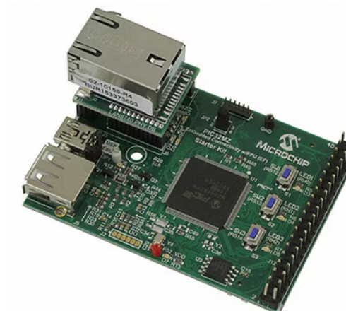
Figure 3: The Microchip Technology DM320007 compact starter kit supports the development and testing of USB and Ethernet applications with the PIC32MZ2048EFH144T-I/PH microcontroller. It includes connectors for USB OTG, USB Host, 10/100 Ethernet, and UART/I2C. Image source: Microchip Technology
