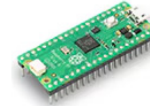
Figure 2: The Raspberry Pi Pico is available in three configurations. Image source: Beningo Embedded Group, LLC
