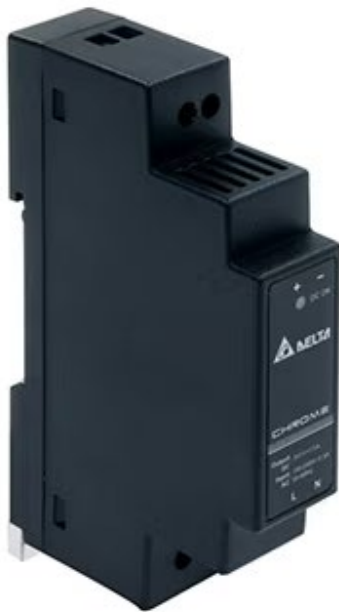
Figure 4: The DRC-5V10W1AZ from Delta Electronics is a double isolated, low-power AC/DC DIN rail power converter, delivering 7.5 watts from a package measuring 91 x 56 x 18 mm. (Image source: Delta Electronics)
