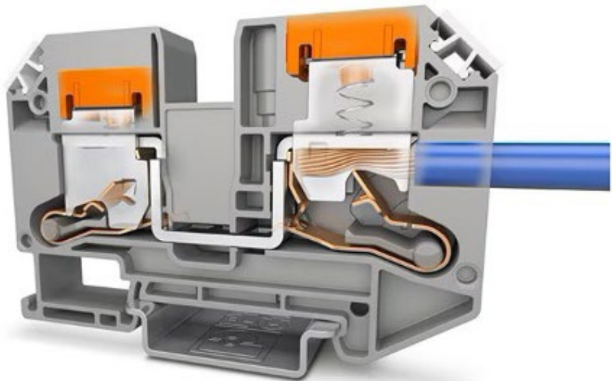
In its factory setting, the pusher is depressed. The orange pusher pops up when the contact spring engages a conductor. (Image courtesy: Phoenix Contact.)
