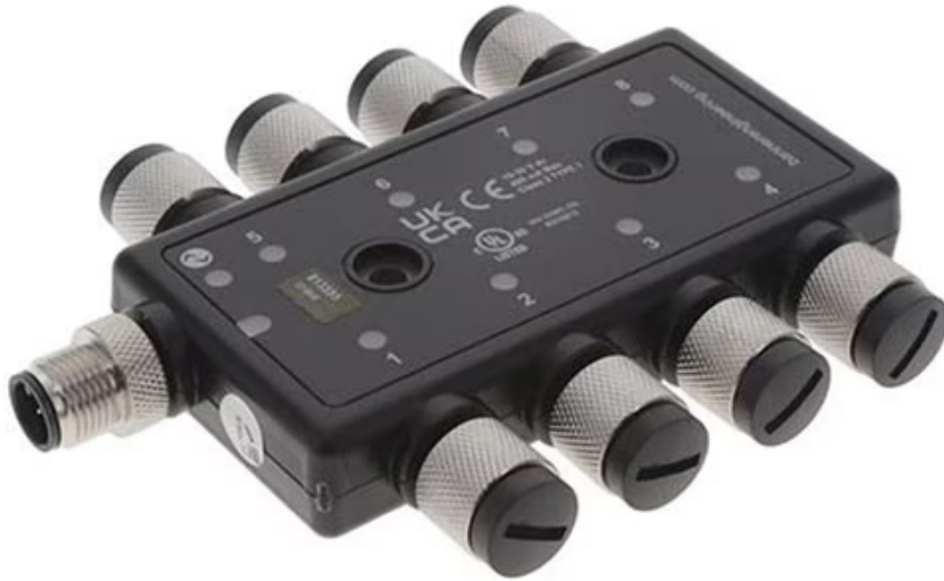
Figure 4: The R95C-8B21-KQ eight-port hub supports both NPN and PNP outputs. Indicator LEDs report port activity and IO-Link status. (Image source: Banner Engineering)
