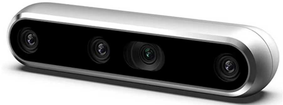
Figure 4: This module includes stereo depth cameras separated by 95 mm, a separate color camera, and an IMU. (Image source: DigiKey)
