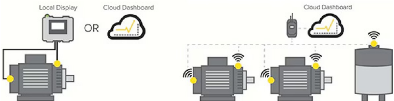
Figure 1: Banner's SNAP ID wired (left) and CLOUD ID wireless (right) EHM gateways have several common features. (Image source: DigiKey)
