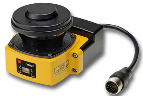
Figure 4: This low-power safety laser scanner supports 70 sets of safety zone and warning zone combinations, making it suitable for AMRs operating in complex or dynamic environments. (Image source: Omron)
