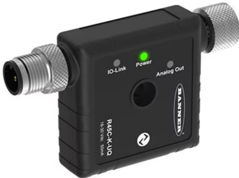
Figure 5: An IO-Link-to-analog output converter produces a current or voltage output controlled by the IO-Link master. (Image source: Banner Engineering)
