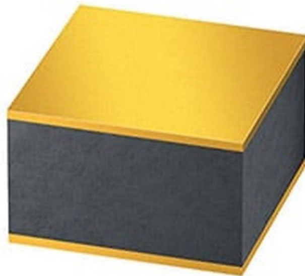
Figure 1: Representation of the NTCWS series device packaging. (Image source: TKD)
