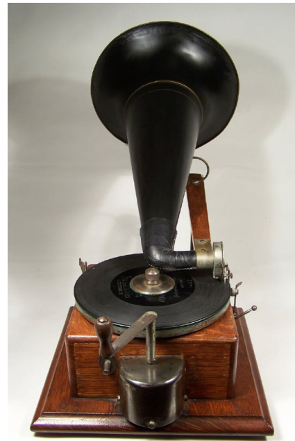
Johnson's Improved Gramophone used a spring-driven motor that mounted to the back of the chassis.
