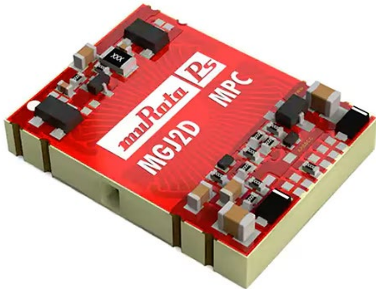
Figure 9: All units in the Murata MGJ2 series of DC/DC converters have the same outward appearance and size, but they are available with a variety of input voltage ratings and bipolar output voltage pairings. (Image source: Murata Power Solutions)
