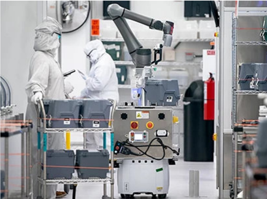
Mobile manipulator working alongside human operators in Analog Devices Beaverton, Oregon chip fabrication facility Image source: Analog Devices Inc
