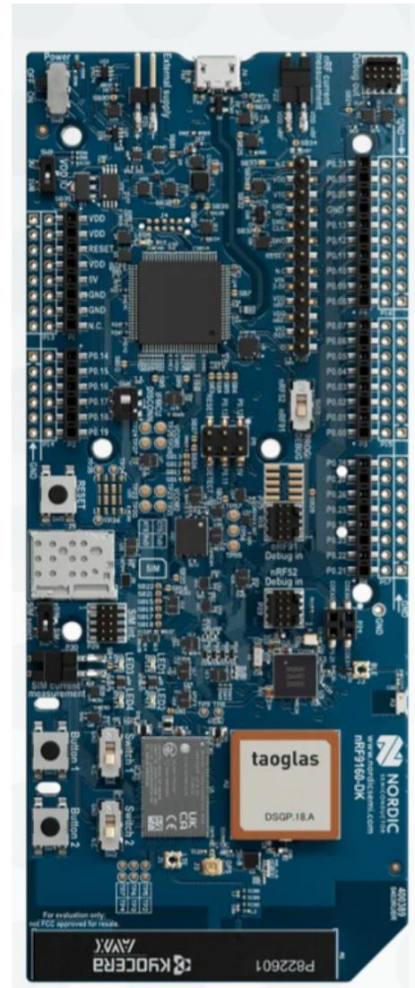
Figure 2: The Nordic nRF9160 cellular IoT development board *Image source: Nordic Semiconductor*
