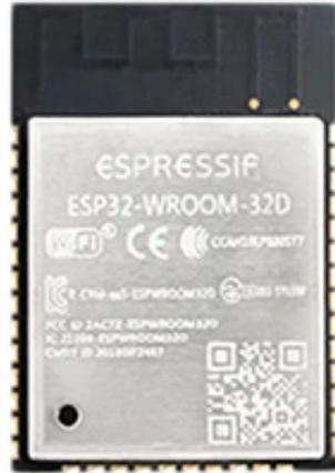
Figure 1. The ESP32-WROOM-32D module runs at speeds up to 240 MHz and contains 8 Mbytes of onboard SPI flash. [Credit: Espressif Systems](#)
