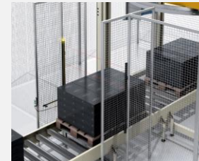
Muting - Temporarily bypass safety light curtain to allow material to be conveyed
