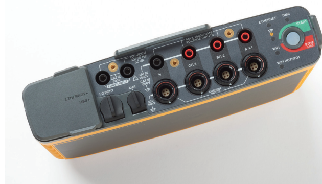
The Fluke 1748 Three-Phase Power Quality Recorder is one of the tools that can be used to help detect voltage unbalance. In reality, voltage differences between phases vary as loads operate. However, motor or transformer overheating, or excessive noise or vibration, can merit troubleshooting for voltage unbalance.
