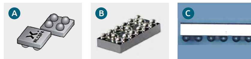
Figure 12 | Examples of wafer level chip scale packages. A WLCSP4 package outline A , a WLCSP15 package with the solder balls on the contact side and the bare silicon body B and a WLCSP15 package with the optional back side coating mold foil C
