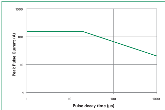
Figure 1: Non-repetitive Peak Pulse Current vs. Pulse Time
