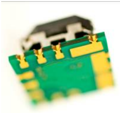
Fig 2: Underside view of the Okami OKL PoL DC/DC converter showing iLGA cutouts that allow easy access for visual inspection as well as test probe access to all pads.
