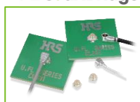
U.FL Stacking Height : 2.5mm Max. Applicable Cable : 0.81/ 0.95/1.13/ 1.32/1.37mm Frequency : 0-18GHz Max.
