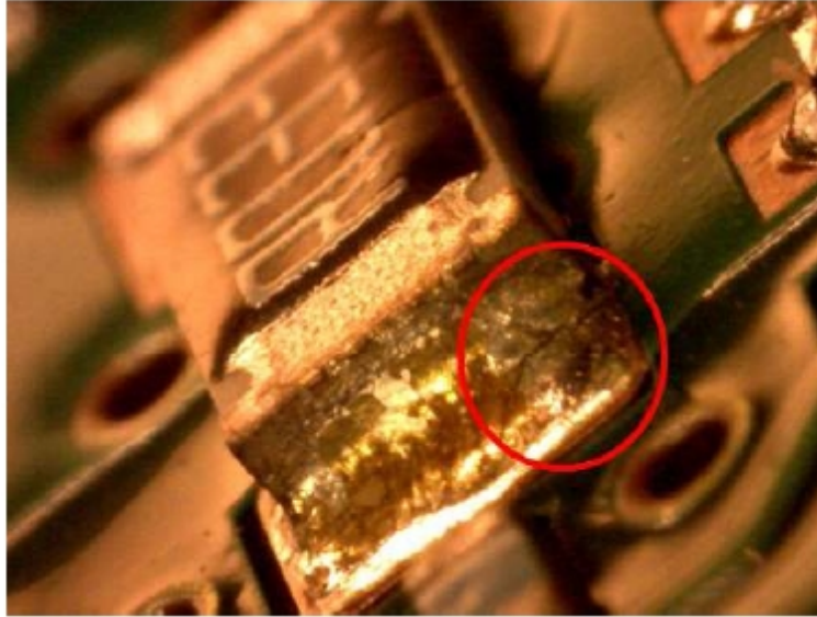
Figure 1 , 2512 size chip resistor showing cracking at the solder joint. (1)
