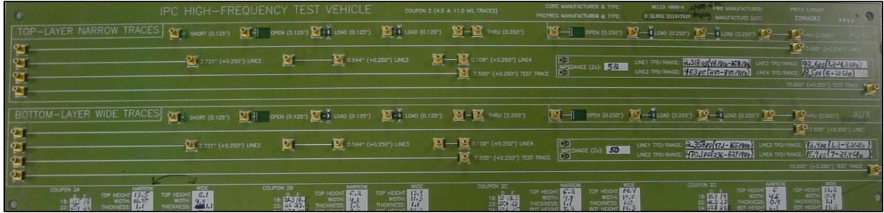
Figure 15: Printed Circuit Board Dielectric Validation Example – Nelco 4000-6 FR4
